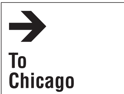
Sign Type 5.4 Used to identify the platform from which to board trains that are headed to Chicago
