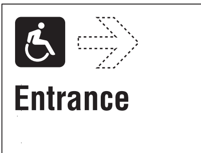
Sign Type 5.19 Used to identify and direct disabled commuters to accessible entrances (add arrow for directional sign)
