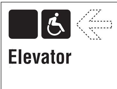
Sign Type 5.18 Used to identify and direct disabled commuters to elevators (add arrow for directional sign)
