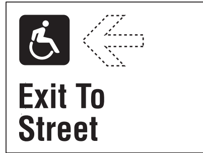
Sign Type 5.21 Used to identify and direct disabled commuters to accessible exits to streets (add arrow for directional sign)
