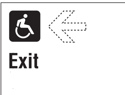
Sign Type 5.20 Used to identify and direct disabled commuters to accessible exits (add arrow for directional sign)
