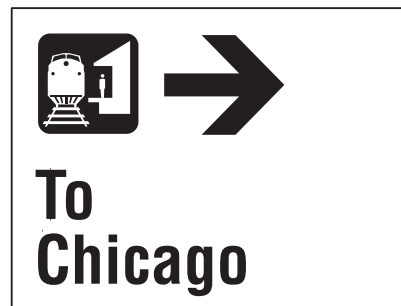
Sign Type 5.6 Used to direct passenger to the platform from which to board trains heading toward Chicago generally mounted in locations where stations and platforms are not visible
